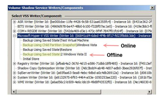
When using the "Backup Using Child Partition Snapshot" method (online), the Hyper-V VSS writer will interface with the Volume Shadow Copy service that is running inside the guest machine (via the installed Hyper-V Integration Services) and create a "live" snapshot. Hence the virtual machine does not need to be stopped and saved at all.
