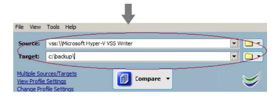
3. ViceVersa will select all files from the Hyper-V VSS writer, create a snapshot using the Volume Shadow Copy service, and copy all the required files to the target (you need to select the Backup or Replication method)
