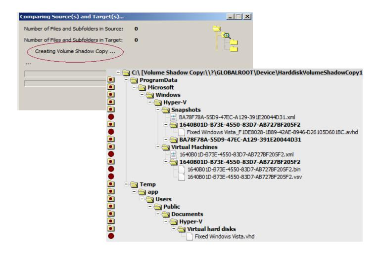
Important Note: When an individual virtual machine is selected for backup, ViceVersa PRO will involve only that specific machine in the Volume Shadow Copy snapshot creation. This means a fast and efficient backup, because the other virtual machines are not saved and are not involved in the snapshot creation at all (which requires additional time and resources). Unlike other general backup applications, ViceVersa PRO can focus on backing up only the selected machine.
